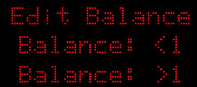
Shift balance in the direction of either speaker in .5dB increments up to a total of 6dB difference - Values are 1-12 where 1 equals .5dB and 12 equals 6dB
