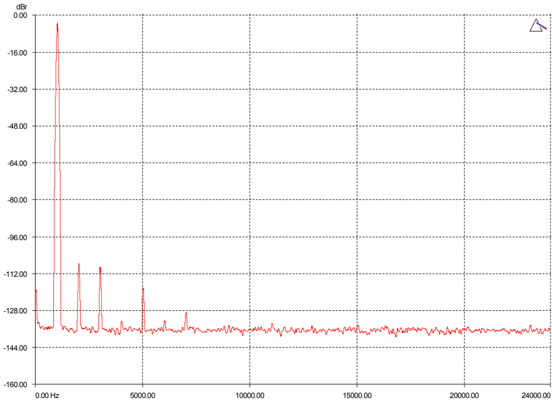
Figure 2. Dac3 0dB 1KHz Sine, 10nS jitter at 10KHz on input data.
